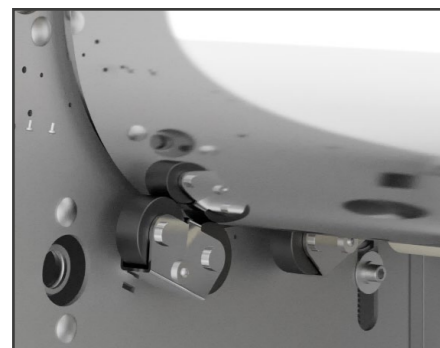
Cylinder Floating Support System.
